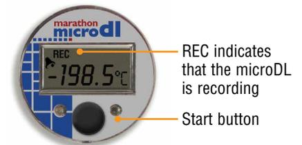
The microDL can now be placed where you want to record the temperature.
